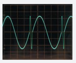
Frequency shifting on alternate cycles.
